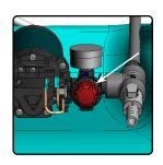
**10)** If the pump is pulsating irregularly, you can adjust the pump pressure setting by turning the set screw in the end of pump. Turn clockwise to increase pump pressure and counterclockwise to decrease pump pressure.
