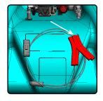
**3)** Mount the hose holders on either the front or the back of your sprayer using the provided holes in the tank with phillips head screws.
