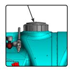
**6)** Before running your pump make sure the regulator is fully open to avoid premature wear or damage to the pump. Turn counterclockwise to open.
