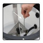
**4)** Prime pump by removing top plug from pump and filling with water.
