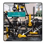
**7)** To properly dissolve dry chemical and increase mixing quality, turn off all valves, and turn on the agitation valve after adding your chemical to the tank.
