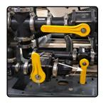
**3)** Open the main valve. This will allow liquid to flow from water source to pump. Ensure all other valves are in closed position.
