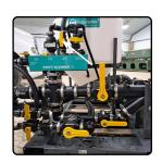
**10)** This unit comes equipped with a spike valve. The purpose for this is if all the valves are closed and the pump is running, this will relieve the pressure off the lines.
