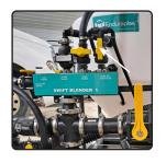
**8)** If you got the optional flow meter, connect the camlock connector on the linch flowmeter pipe to the linch port on swift blender (you can draw from two chemical totes). This allows you to measure the amount of chemical from tote to applicator.
