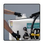
**6)** To empty the mixing tank, close the main valve, open the venturi valve, switch the 3-way source valve to draw from the mixing tank. Then start your pump.
