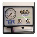
**8)** To make sure your solenoids have power, switch the 3 valve controls on and off listening for the valves to click open and shut on the sprayer. This will ensure valves are powered and operating.
