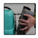
**4)** Wrap threads on spigot with sealant tape and thread spigot into tank.
