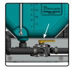
3) Before starting PTO, make sure the pressure regulator is fully open (counterclockwise) to avoid premature wear or damage to the pump. This will allow liquid to flow from pump and return back to tank. Pump should prime automatically. (Electric solenoids, refer to page 16.)
