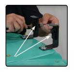
**3)** Wrap hose around and insert gun into clips.
