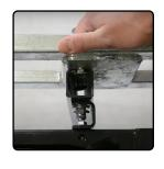
**4)** When the boom is set to desired height, tighten the hardware listed in steps 2 & 3, making sure the square neck on the carriage bolt is fully inserted through the slot.
