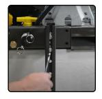
3) To install your boom to the brackets, loosen the carriage bolts on the boom (leaving nuts and washers on bolts). Align carriage bolts with quick attach brackets and slide them into the bracket slots, then lower the boom down to desired height.
