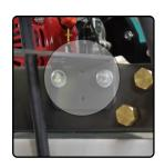
**10)** Hook up hoses, with female brass fitting, from boomless nozzle to male brass ports on back of sprayer. Make sure washer is installed in female fitting to prevent leaking.
