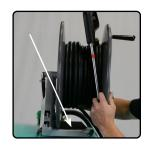
**2)** Insert four 3/8" x 3/4" bolts with 3/8" flat washers and lock washers through hose reel into inserts in tank. Secure tightly.
