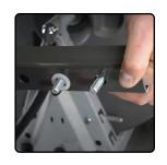
2) Connect the brackets by sliding the 3/8" x 1" bolts through the C-bracket on unit and install 3/8" washer and 3/8" lock nuts loosely. Leaving these bolts loose allows the bracket to adjust in step 3.
