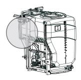
1) Connect controller bracket using four 1/4" x 3/4" bolts, four 1/4" flat washers, and four 1/4" lock washers.
