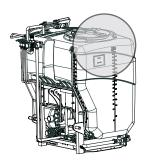
**1)** Attach the 2 brackets to the tank using two 3/8" x 3/4" bolts, two 3/8" flat washers, and two 3/8" lock washers.
