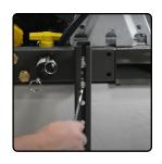
6) Take the feed hoses from boom and connect to male brass hose fittings on spray unit. Hook hoses up to the appropriate section control; 12', 20' and 30' booms have 3 hose hookups and boomless nozzle has 2 hose hookups.
