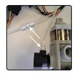
**6)** This unit comes with power wires that you will either need to add gator clips to or wire directly to a power source. If gator clips are used, connect to battery; red to positive and black to negative. Make sure there is no place for it to get cut or pinched.
