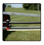
2) Measure Appropriate Travel Distance Mark the distance with flags or between fence posts. A tape measure capable of measuring farther than 200 ft. will make this step easier.
