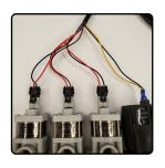
**4)** There are 2 wires in this harness running back to the solenoid kit that plug into the electric valve, yellow is positive and green is negative.
