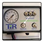
**11)** Once you have reached desired pressure, test the spray boom by turning on the Left, Center, and Right control switches. This will open the electric valves allowing flow out boom sections. (Left Center and Right)
