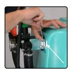
**3)** Lubricate and insert hose into provided grommet in tank. Push hose about 4" into tank through gommet.
