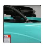
**10)** With sprayer pump running, increase your pressure to desired amount by holding up on pressure control toggle switch; hold up for a couple seconds, then release. At 0 PSI, liquid should be returning into the top of tank. As the pressure goes up, the return to tank will slow down and pressure to boom will increase.
