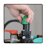
**6)** Once you have set your desired pressure, test the spray boom by turning on Right, Center, and Left section controls. When controls are in the up position, the sprayer boom should be engaged.
