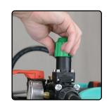
**4)** If liquid is not flowing into tank through the return line, there may be an airlock in the line and you may need to prime the pump. Remove plug from back of pump, allowing air out of the line. When liquid starts to flow, reinsert plug and pump should be primed.
