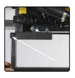
**4)** Slide the second bracket onto the other end of the stand and mount it to the sprayer frame. Then tighten all bolts. Repeat on the other side of the frame to complete stand.
