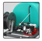
**3)** Disconnect the suction hose from pump and attach it to the top outlet.
