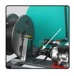
**4)** Attach 25' draft hose from Quickfill™ draft kit to suction port on pump (bottom). Ensure water is present in the bottom of the pump housing to allow unit to self prime. If pump needs to be primed, repeat step 1 of priming pump.
