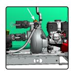
**2)** Before starting your engine, make sure the drain plug and prime plug are tightened securely and properly holding the seal O-rings in place.
