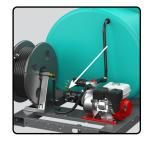
**7)** Start engine and operate until tank is full. We recommend opening tank lid while filling.
