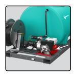
**8)** When tank is full, turn engine off and close suction valve between pump and tank.
