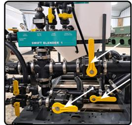
**7)** To properly dissolve dry chemical and increase mixing quality, turn off all valves, and turn on the agitation valve after adding your chemical to the tank.
