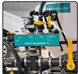
**8)** If you got the optional flow meter, connect the camlock connector on the 1inch flowmeter pipe to the 1inch port on swift blender (you can draw from two chemical totes). This allows you to measure the amount of chemical from tote to applicator.
