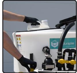
**6)** To empty the mixing tank, close the main valve, open the venturi valve, switch the 3-way source valve to draw from the mixing tank. Then start your pump.
