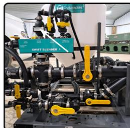
**11)** This unit comes equipped with an auxiliary rinse port. This is a fresh water supply in case any spills need to be rinsed.
