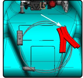
**3)** Mount the hose holders on either the front or the back of your sprayer using the provided holes in the tank with phillips head screws.
