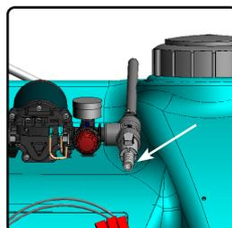
**2)** Pour small amount of anti-freeze into tank, then turn pump on and hold trigger on gun. Spray until anti-freeze comes out of spray wand tip. Then, power pump off.
