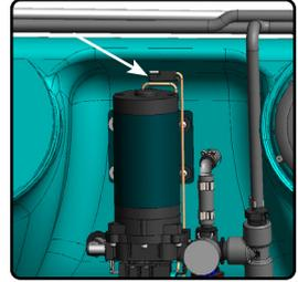
**2)** If you choose to use battery clip wire harness, connect the 2 prong plug on wire harness to the 2 prong plug on pump and attach clips to battery. Red clip on positive post and black clip on negative post.
