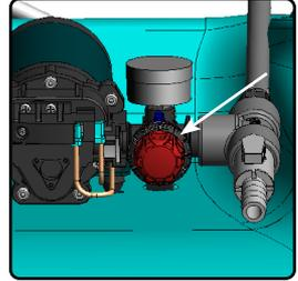
**10)** If the pump is pulsating irregularly, you can adjust the pump pressure setting by turning the set screw in the end of pump. Turn clockwise to increase pump pressure and counterclockwise to decrease pump pressure.
