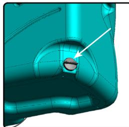
**2)** After draining the tank, rinse the inside of the tank out by spraying clean water with water hose.
