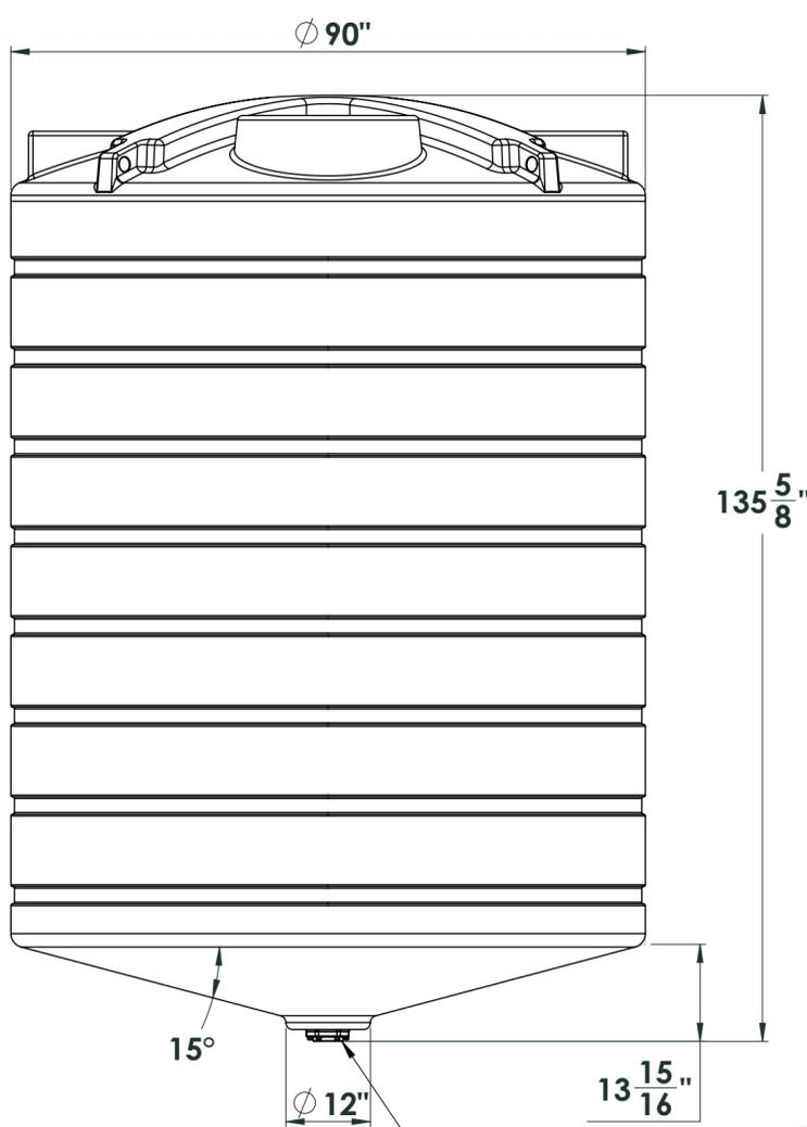
3 inch bolted - bottom drain fitting
