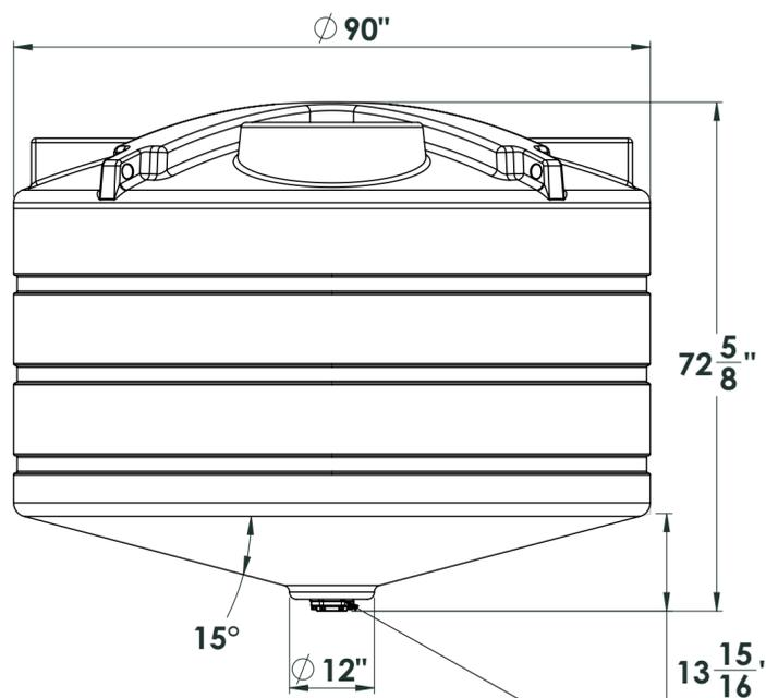
3 inch bolted - bottom drain fitting
