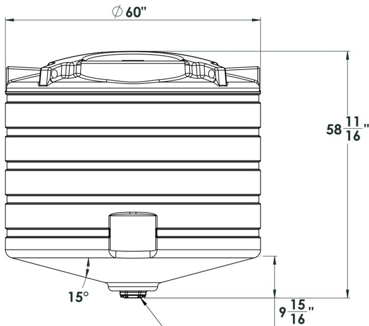
3 inch bolted - bottom drain fitting
