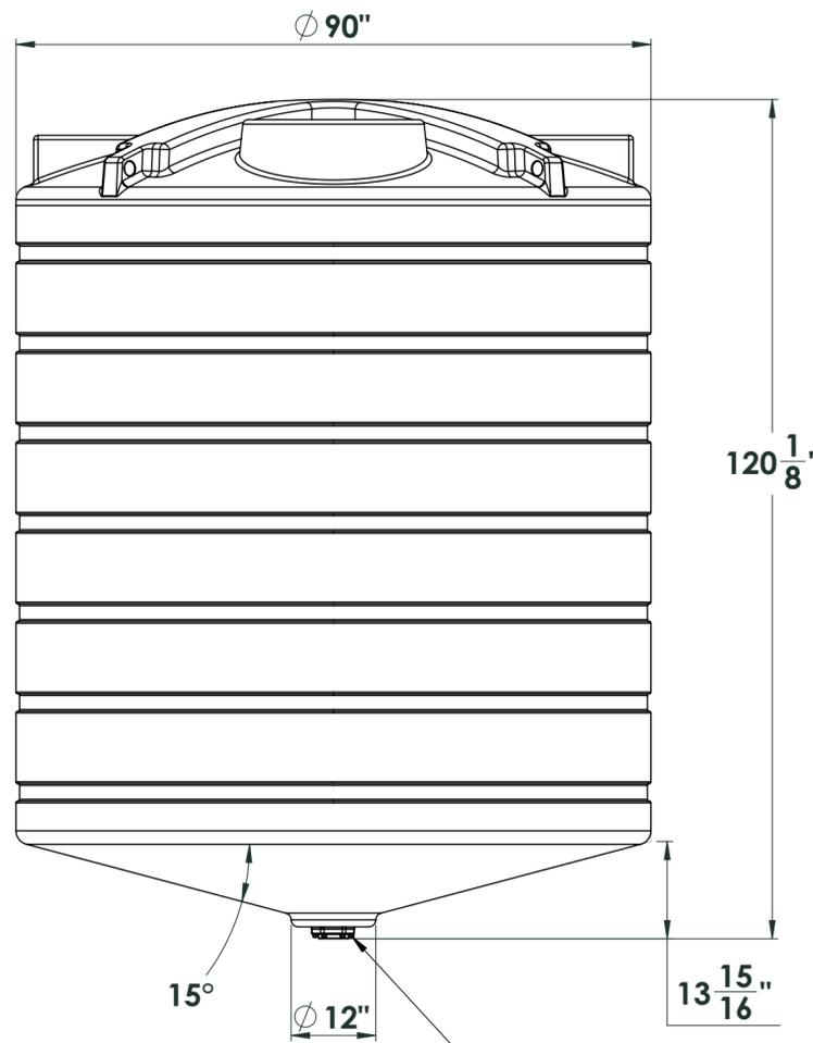
3 inch bolted - bottom drain fitting
