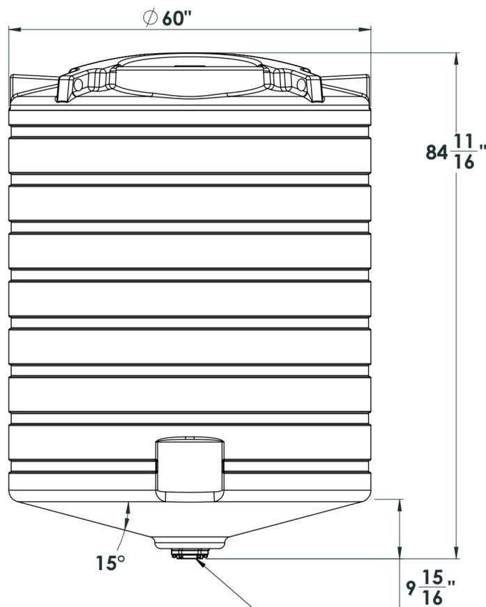
3 inch bolted - bottom drain fitting
