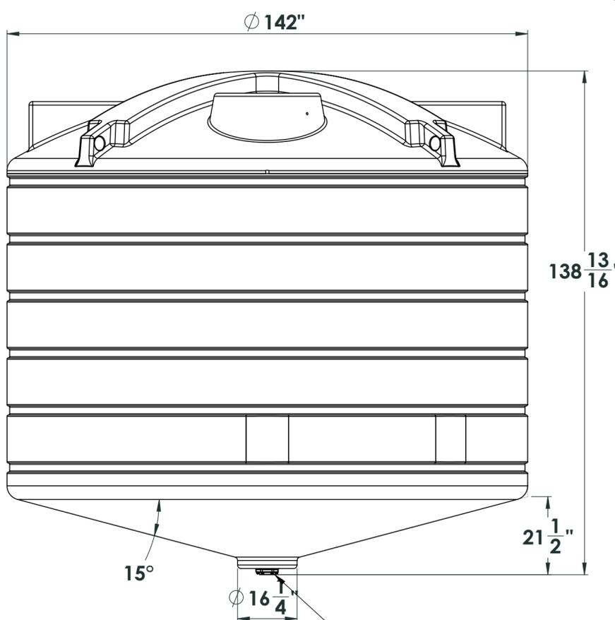
3 inch bolted - bottom drain fitting
