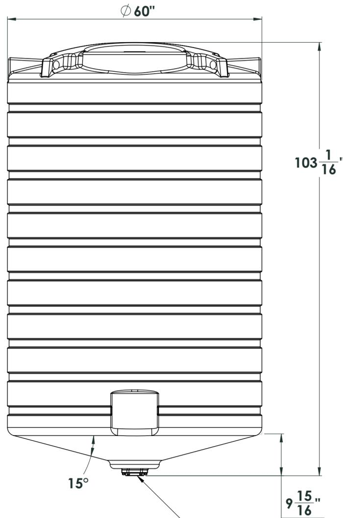
3 inch bolted - bottom drain fitting
