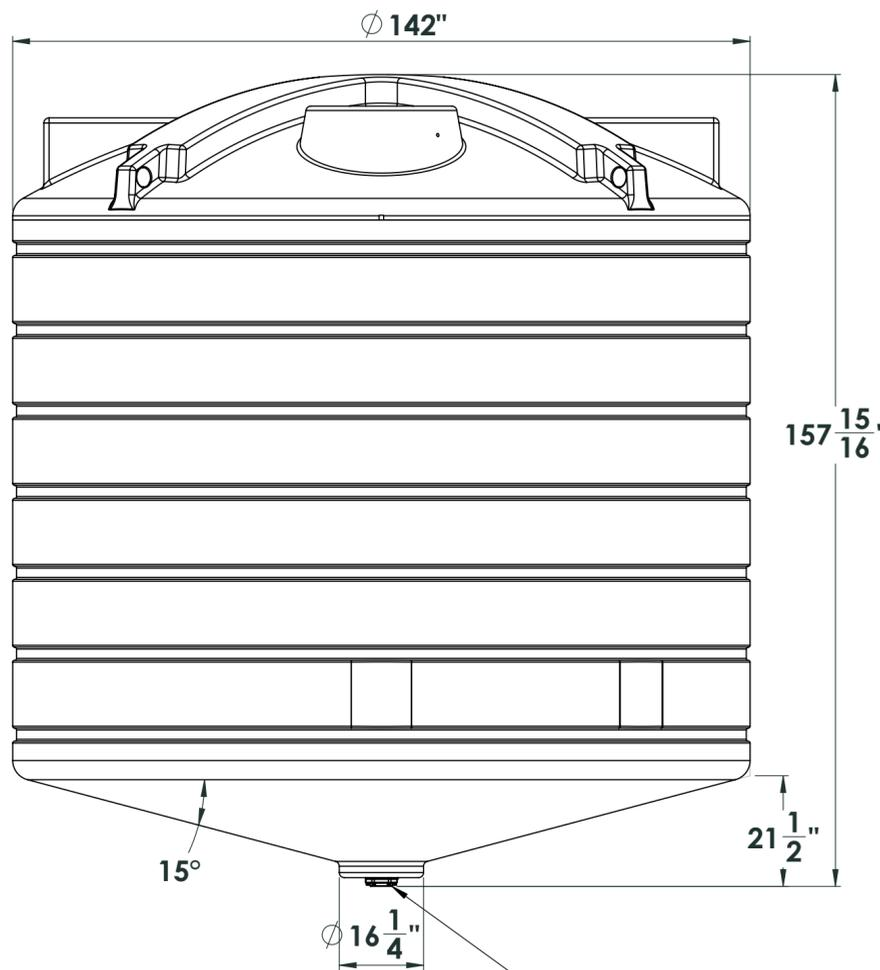
3 inch bolted - bottom drain fitting
