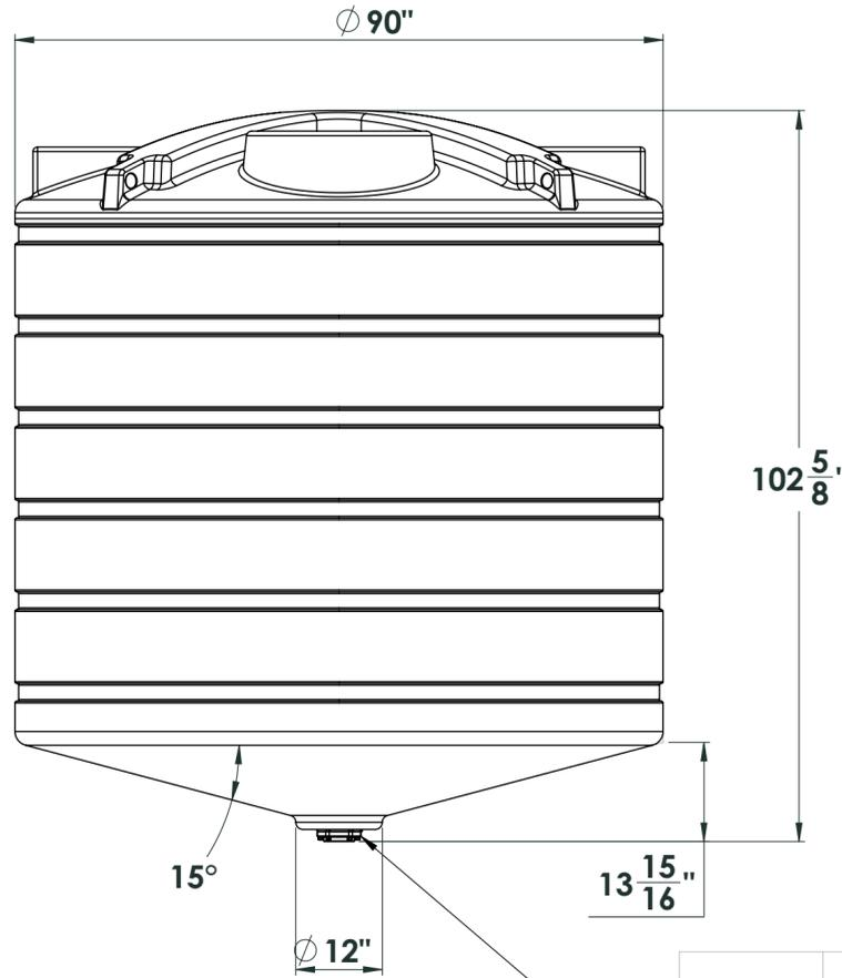
3 inch bolted - bottom drain fitting
